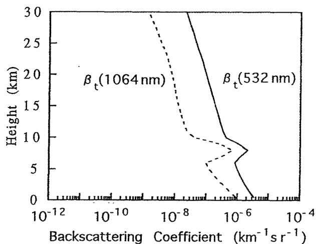
Fig. 3. The total backscattering coefficients for 1064 nm and 532 nm laser wavelength.
