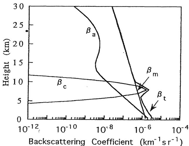
Fig. 2. The atmospheric model employed in signal simulations.  $\beta_m$ ,  $\beta_a$ , and  $\beta_c$  are the backscattering coefficients of molecules, aerosols, and clouds respectively.  $\beta_t$  represents the total backscattering coefficient. Calculations were made for 532 nm laser wavelength.
