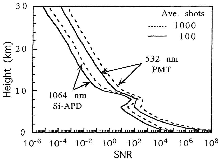
Fig. 5. The range dependence of signal-to-noise ratio for both wavelengths. The SiAPD is assumed to have an avalanche gain of 100 and quantum efficiency of 10%. The NEP is  $8 \times 10^{-14} \text{ W Hz}^{-1/2}$ . The PMT has a current amplification gain of  $1 \times 10^7$ . The dark current is 3 nA, sensitivity is 74 mA/W and quantum efficiency is 10%. Calculations are also based on night time operation.
