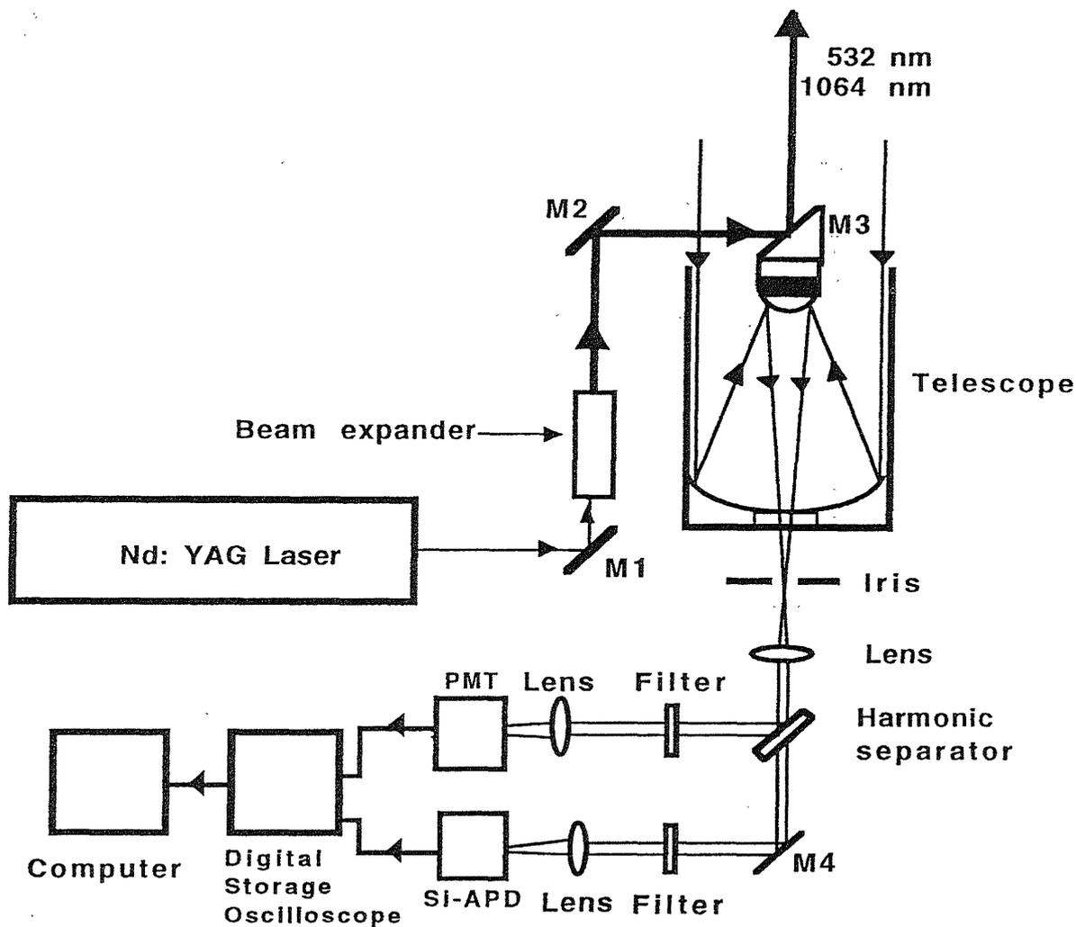
Fig. 1. Block diagram of the Mie lidar system.
