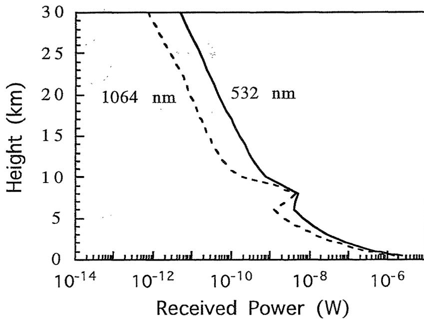
Fig. 4. The calculated received signal for both wavelengths based on the model atmosphere and the system parameters given in Table 1.
