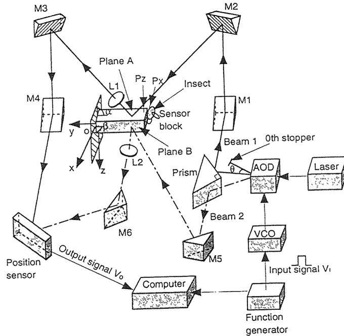
Fig. 1 Configuration of the TSC system
