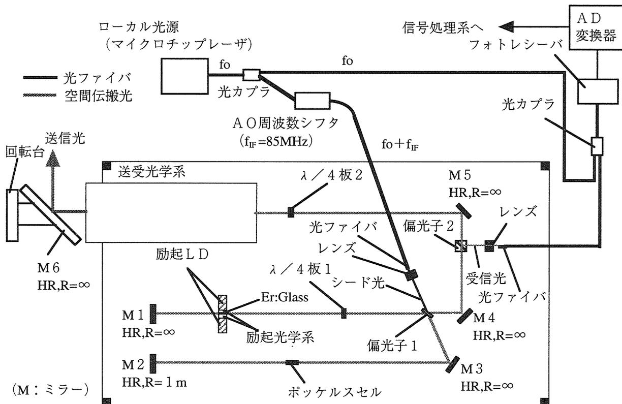
Fig.1 Block diagram of the coherent lidar.
