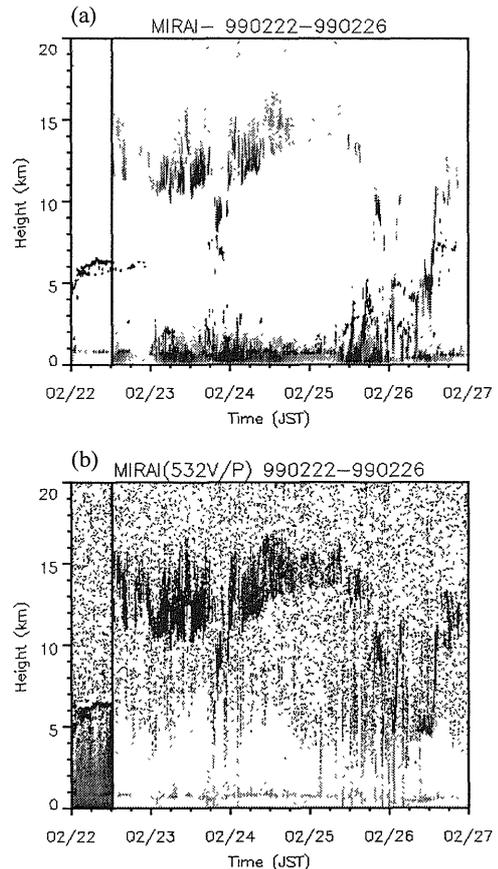
Fig.3 Time-height indication of (a) lidar backscatter intensity and (b) depolarization at 532nm, observed between February 22 and 27, 1999.
