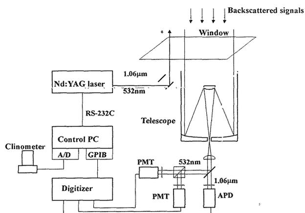
Fig.1 Shipborne lidar system installed in the container.
