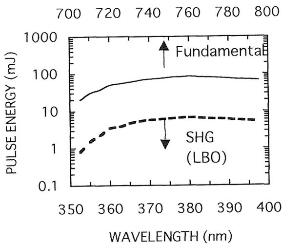
Figure 2. The tuning curve of the second-harmonic wavelength.
