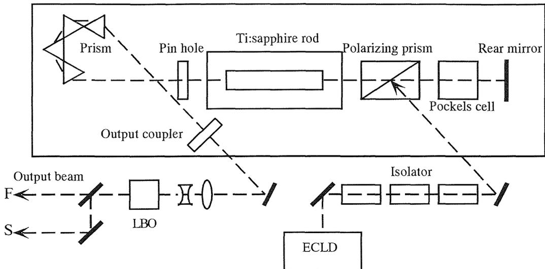
Figure 1. The schematics of flashlamp pumped Ti:sapphire laser seeded by a external cavity laser diode.
