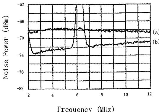
Fig. 2 Noise power spectrum of (a) the shot-noise level and (b) the intensity difference between twin photon beams.
