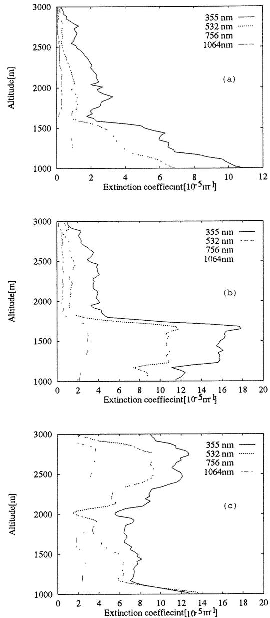
**Fig. 1** Results of the present method to the multi-wavelength lidar data measured at (a) 1 June 1999, 14:50, (b) 9 August 1998, 13:00 and (c) 11 April 1998, 12:45.
