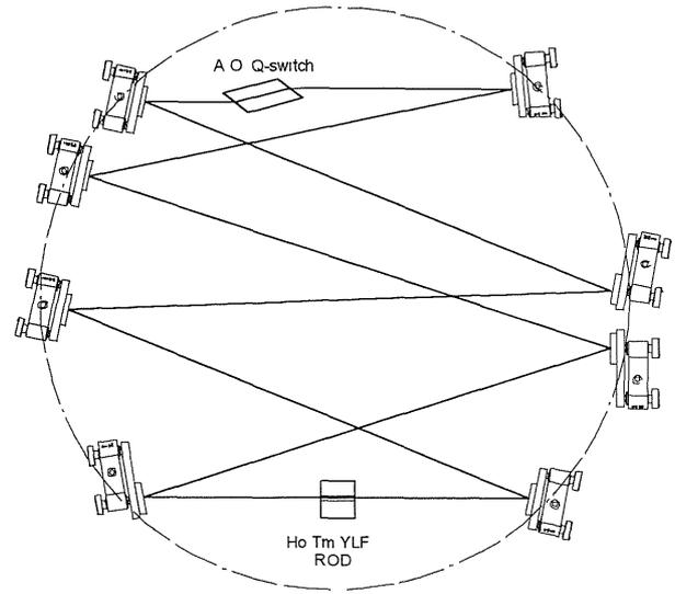
Figure 3. Power oscillator with folded cavity to fit into shuttle hitchhiker canister.
