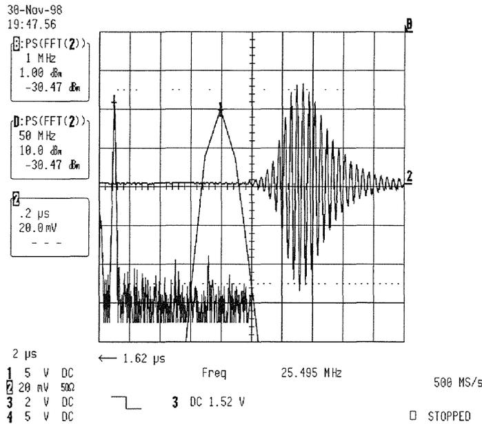
Figure 6. Injection-seeded Q-switched operation
