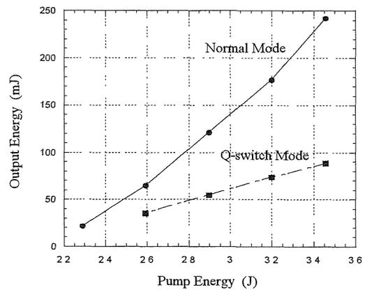
Figure 4. Output energy of the folded resonator as a function of diode pump energy for a rod temperature of 20 degrees C.
