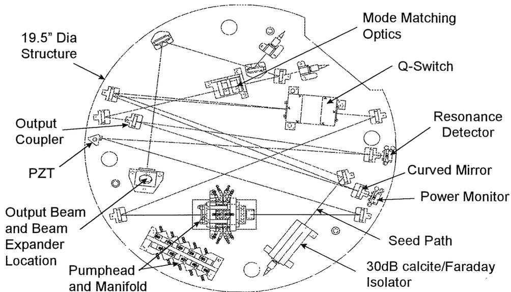
Figure 5. Optical layout of slave oscillator assembly
