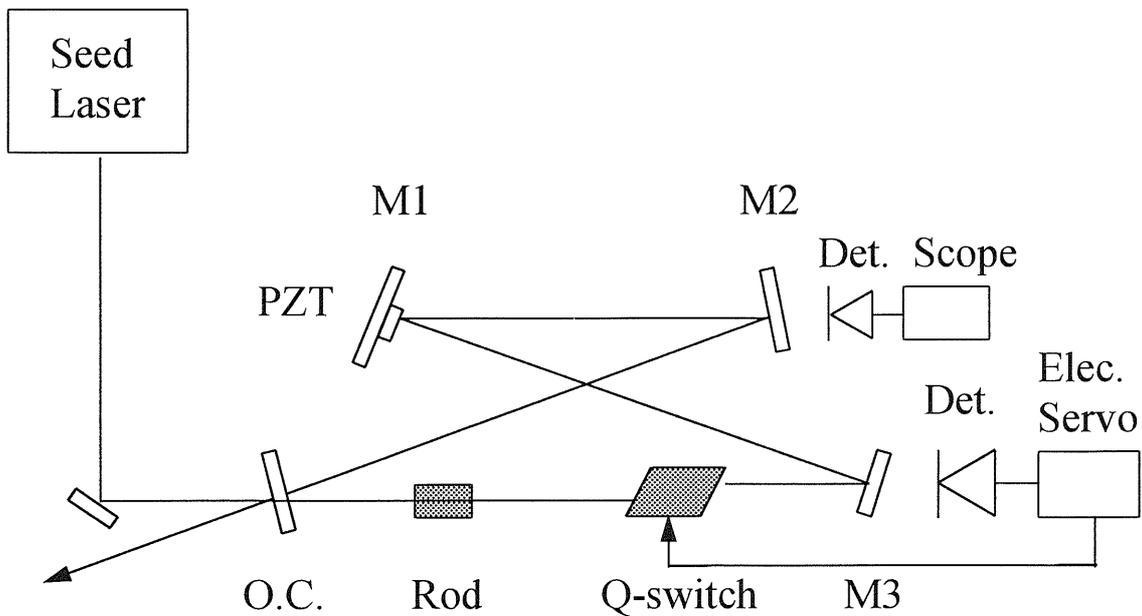
Figure 1. Schematic of injection-seeded Ho:Tm:YLF laser system
