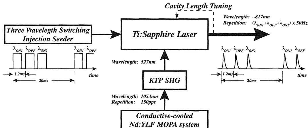
Fig. 1 Block diagram of the developed Ti:Sapphire laser system
