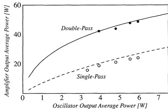
Fig. 3 The amplifier output average power as a function of the oscillator average power (experimental data by signs and a theoretical results by lines).
