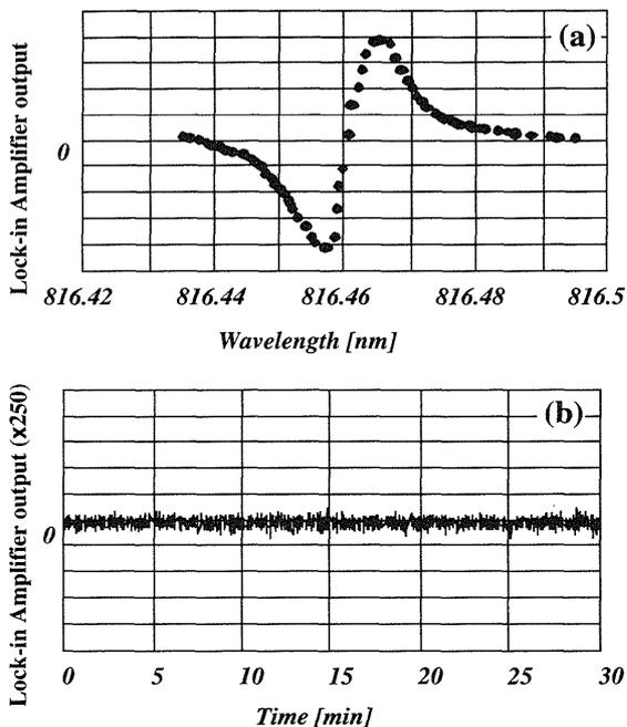
Fig. 5 Fast derivative signal (a) and the wavelength stability of ON2 (b). The stability is  $\pm 0.0017$ -pm.
