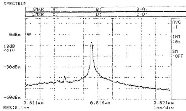
Fig. 6 Output spectrum of the ON2 with the polarization switch. More than -30dB suppression of the ON1 power and the OFF power was obtained.
