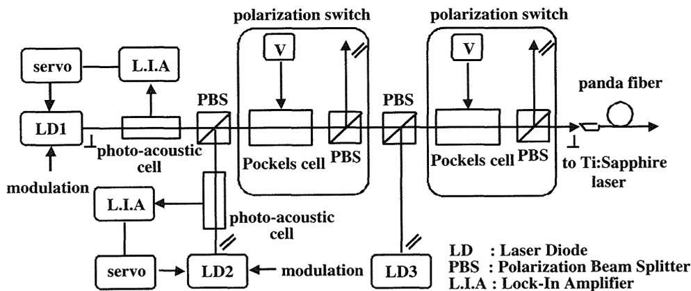
Fig. 4 Diagram of the injection seeder.
