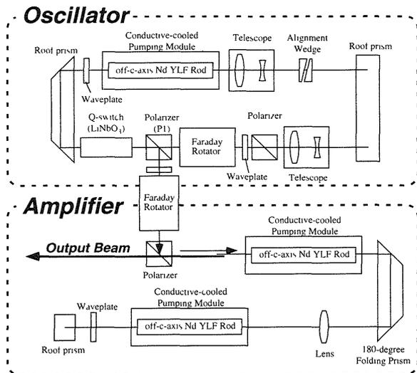
Fig. 2 The conductive-cooled Q-switched Nd:YLF MOPA system.
