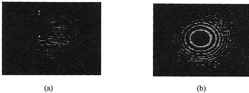
**Figure 2** The Fabry-Perot interference fringe pattern of the pulse dye laser. (FSR=1.5GHz)
