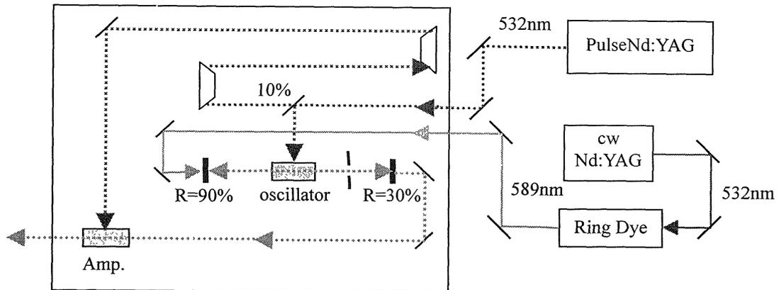
**Figure 1** The block diagram of the injection-seeded dye laser system.
