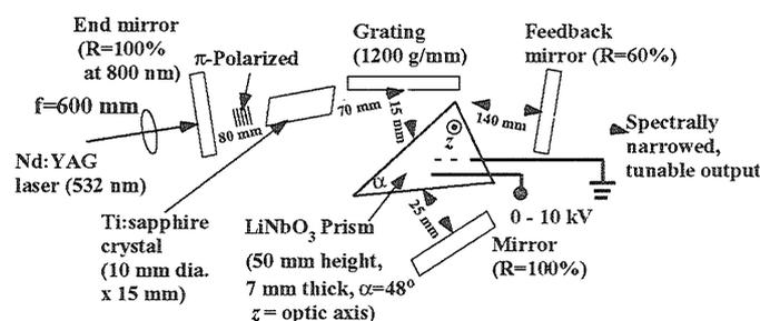
Figure 1: Experimental setup.
