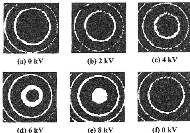
Figure 2: Fabry-Perot interferograms of  $\text{Ti}^{3+}$ :sapphire laser at different electro-optic voltages. (a) Without, (b to e) with the application of voltage to the prism, and (f) when the voltage is reduced to zero. Free spectral range =  $1.66 \text{ cm}^{-1}$ .
