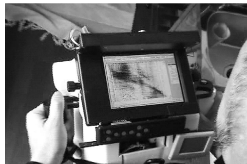
Fig. 6 Visualization of leak from under the carpet.
