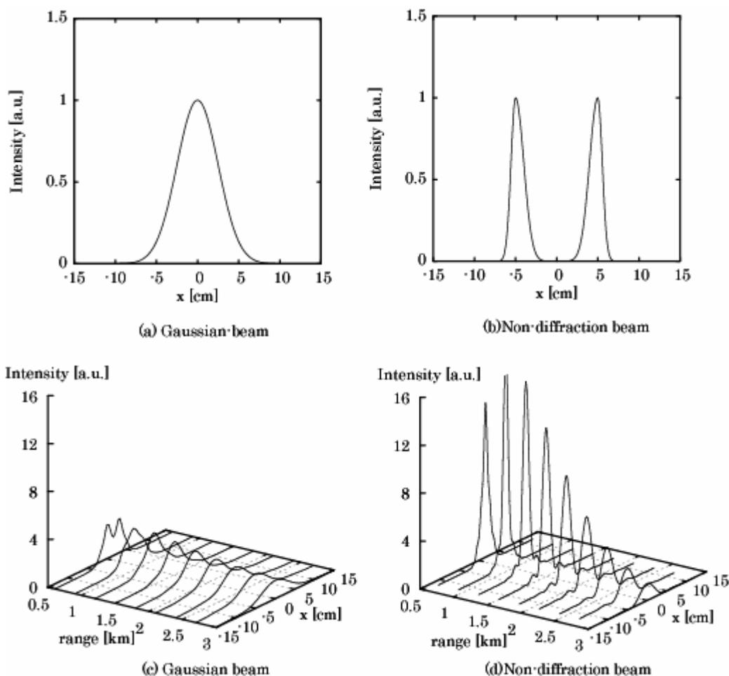
Fig.1 The characteristics of the gaussian and non-diffraction laser beam propagation.
