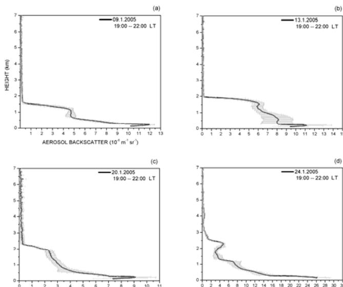
Figure 3. Height profiles of mean aerosol backscatter observed on selected days to show the aerosol backscatter variability shown as shaded lines about the mean aerosol profile.
