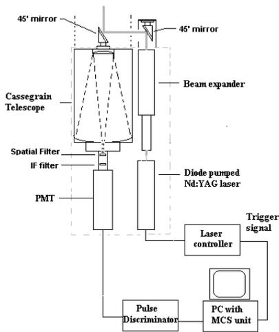
Figure 1. Schematic block diagram of boundary layer lidar (BLL) system
