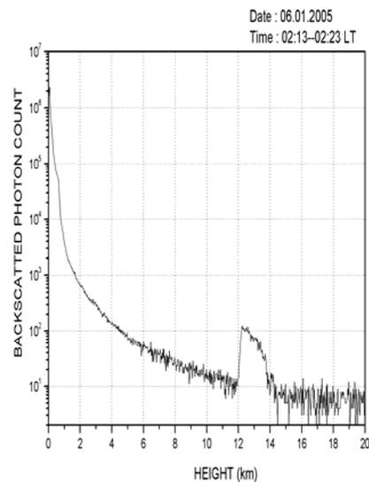
Figure 2. The basic photon count profile from the BLL system, indicating the occurrence of high altitude cloud over the lidar site during the observational period.
