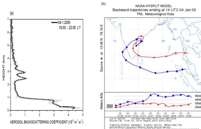
Figure 4 (a) BLL observation of elevated aerosol layer detected on 4 January 2005 over lidar site, (b) A 10-day back trajectories showing the air mass advection from Far East
