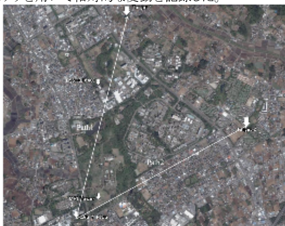
図 2 - The location (36°03.0'N140°07.2'E) included the observation path1 (2.8km) and path2 (2.5km) of the LAS and positions of the in situ measurement. Observation path length (white line) of the LAS positioned on the 8 th floor of the building in the NIES (indicated as the "LAS @ NIES" in this figure) and the positions of the in situ measurement (indicated as TKSC (Li840) and MRI tower in this figure).
