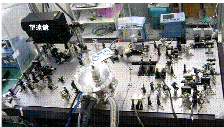
Fig.2 CO2DIAL/Doppler lidar on an optical table
