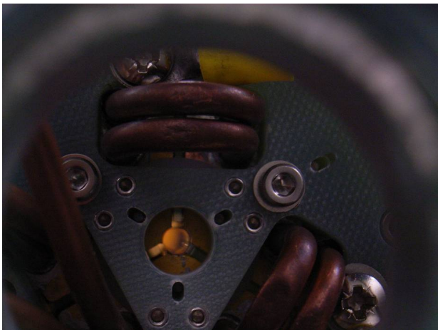
Fig.1 Laser rod pumped from three directions
