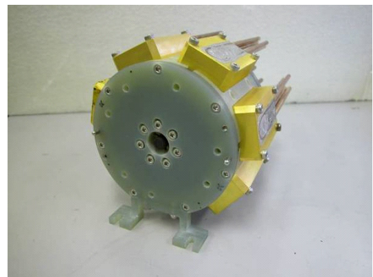
Fig.1 Laser head pumped from seven directions
