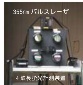
Fig.1 Fluorescence imaging LIDAR
