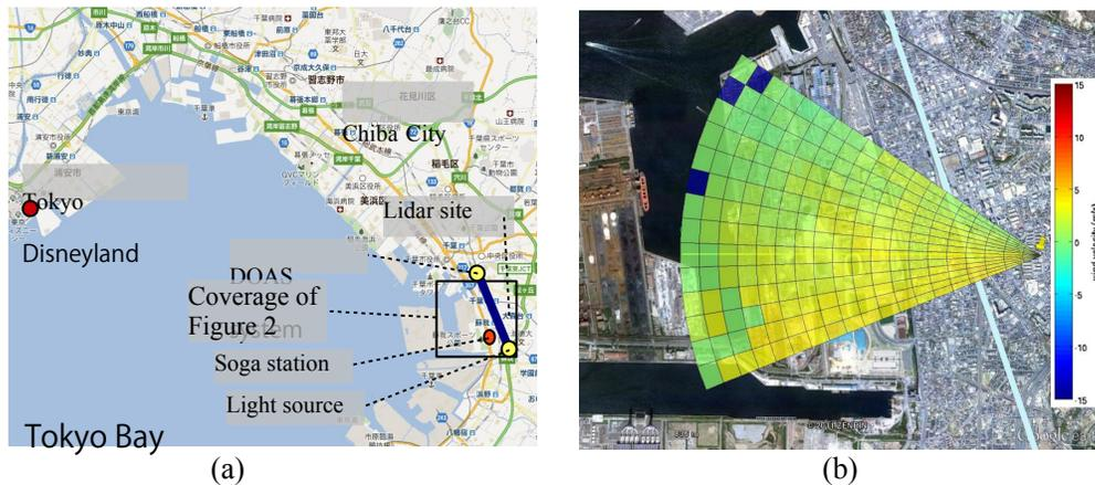
Figure 1 (a) Location of observation site East of Tokyo Bay and (b) Coherent Doppler Lidar area coverage and DOAS light path (blue line).
