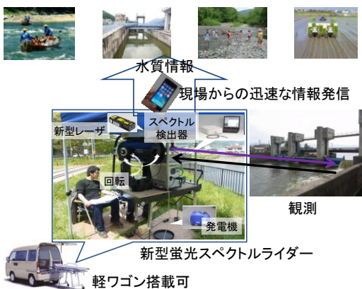
Fig. 1 Concept of LIFS lidar observation
