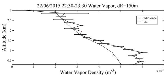
Figure 3. The 1 hour average water vapor density with 150 m range resolution and the radiosonde data.
