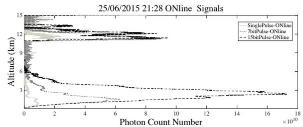
Figure 5. The photon-count numbers of the online signals with single pulse, 7-bit pulse modulation, and 15-bit pulse modulation.
