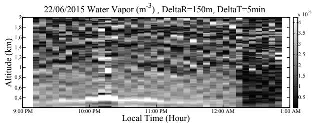
Figure 2. The water vapor profiles observed in nighttime June 22, 2015 with 150 m range resolution and 5 minute time resolution.
