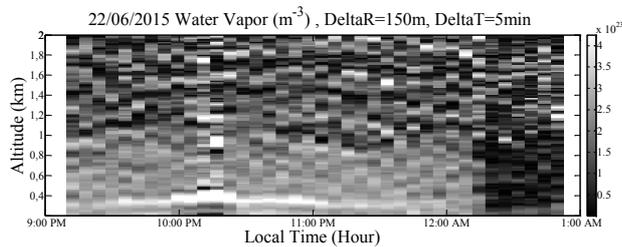
Figure 2. The water vapor profiles observed in nighttime June 22, 2015 with 150 m range resolution and 5 minute time resolution.
