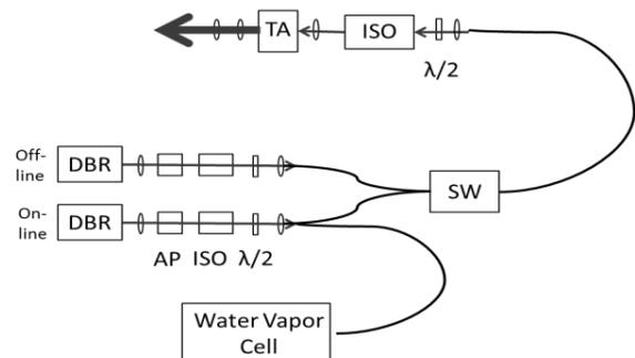
Figure 1. Block diagram of the DIAL transmitter.
