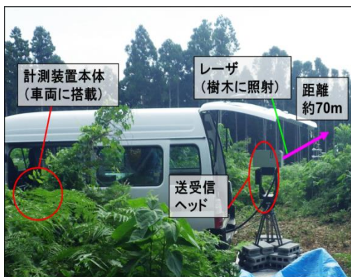
Fig.1 Schematic of experimental setup 1)
