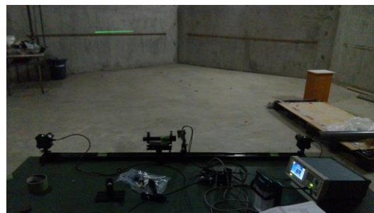
Fig.4 Photo of the scanning laser and two Line CCDs system with curved wall in 8.1m distance
