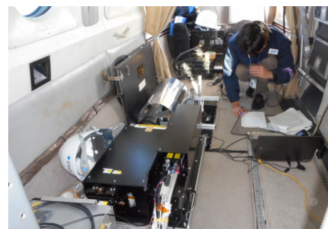
Fig.1 air-borne set-up of vegetation lidar
