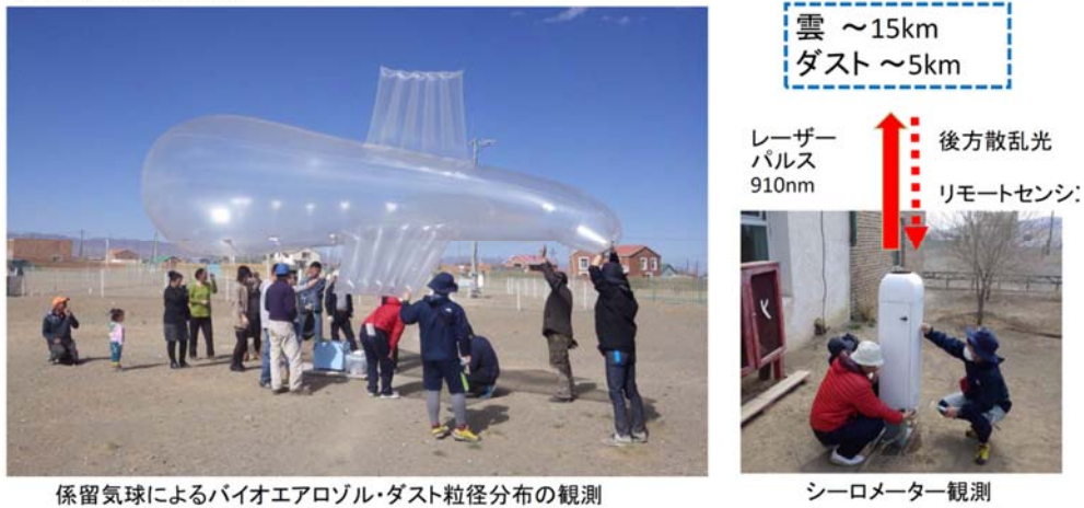
Fig.1 Comparative observation of Asian dust by a dust balloon and ceilometer at Dalanzadgad observatory, Mongolia at 8 LST on 29 April 2016.
