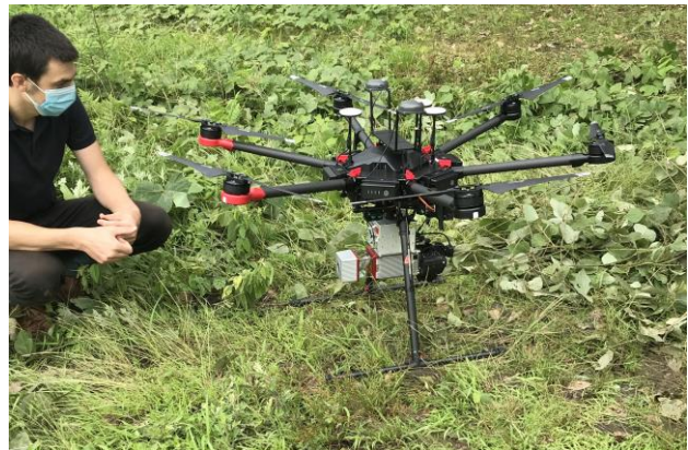
Fig. 1. Photo of miniRANGER attached to DJI Matrice 600 Pro
