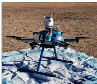
Fig. 2 Photograph of the drone. Air temperature, pressure, and wind sensors are on the top, and the dewpoint sensor is beneath the drone.
