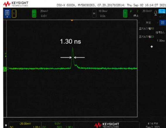
Fig.2 Measured Output Pulse of Microchip Laser@1064nm.
