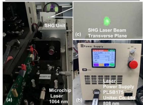
Fig.1 (a)Microchip Laser Head, (b)Laser Power Supply for Pump LD@808nm and (c)Transverse Plane of SHG Laser beam.
