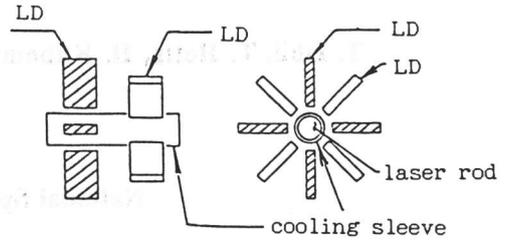
Fig 2. 1-2 Structure for LD pumping
