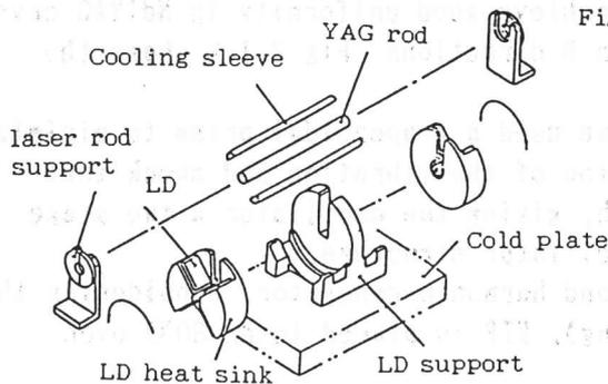
Fig 2. 2-1 The structure of the cooling unit for the laser head
