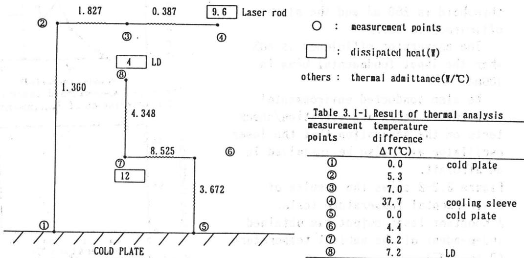
Fig. 3.1-1 Schematic diagram of thermal analysis
