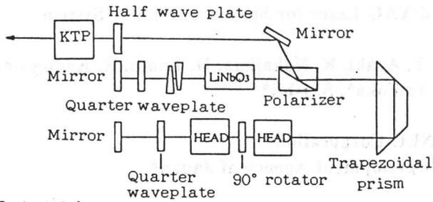
Fig 2. 1-1 Schematic diagram of the laser oscillator
