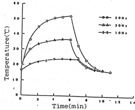
Fig3. 1-3 Results of cooling sleeve temperature measurement
