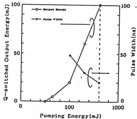
Fig 3. 2-1 Q-switched laser output characteristics of fundamental beam
