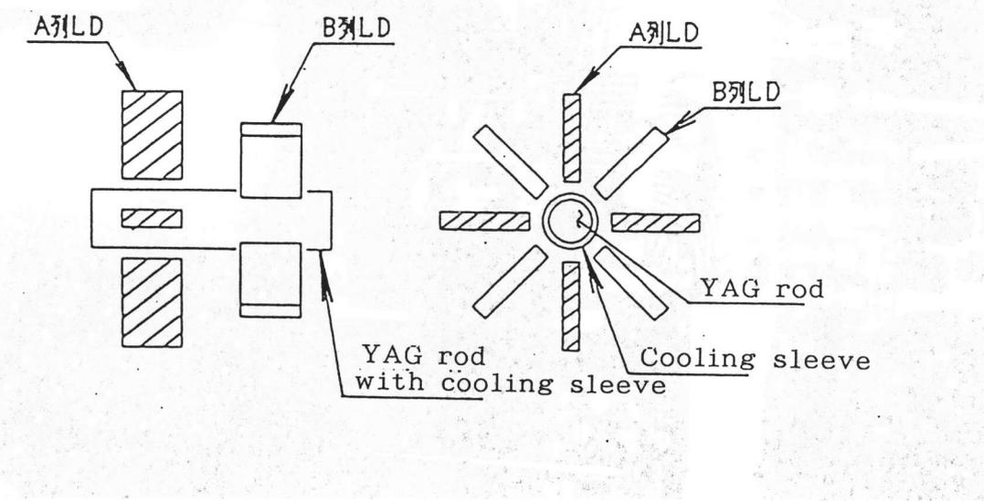
**Schematic diagram of the laser oscillator**
