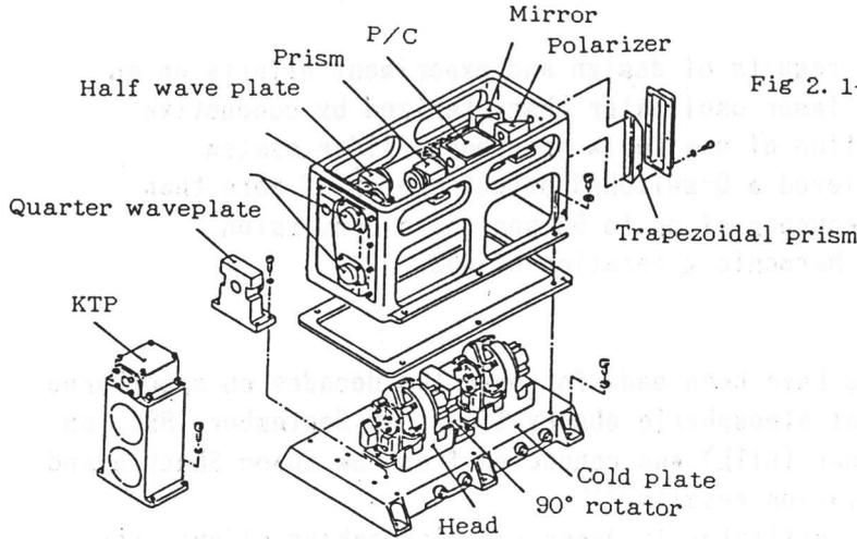
Fig 2. 1-3 The oscillator structure
