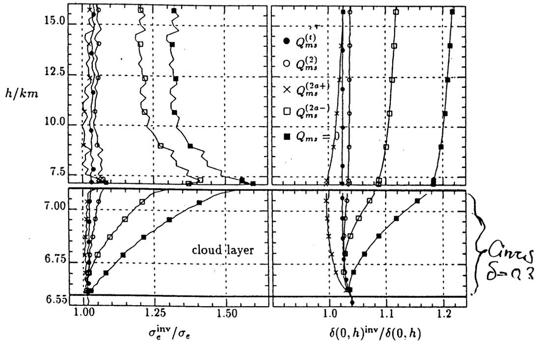
Figure 11: Same as Figure 7, except that the inverted signals were simulated using a ice crystal cloud with phase function No. 1.1 of Table 1 at the height of 7 km with an optical depth 0.3.
