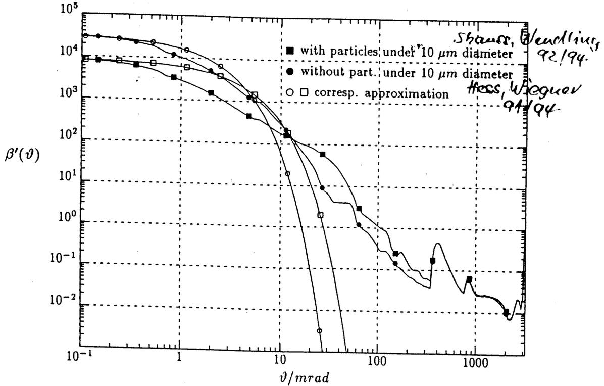
Figure 2: Phase functions for the clouds at the height of 10.0 to 10.5 km with temperature in the range  $-(55 \dots 60)^\circ\text{C}$ . Filled circles: ice crystal cloud without particles under  $10 \mu\text{m}$  diameter according to No. 1.8 of Table 1. Filled squares: ice crystal cloud with particles under  $10 \mu\text{m}$  diameter according to No. 2.2 of Table 2. Open symbols: approximations according to Equations (19) and (20).
