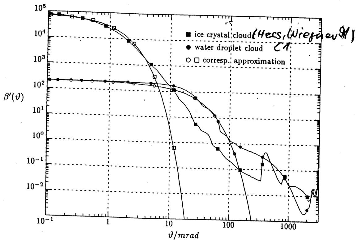
Figure 1: Phase functions for the clouds at the height of 6.6 to 7.1 km with temperature in the range  $-(25 \dots 30)^\circ\text{C}$ . Filled squares: ice crystal cloud according to No. 1.1 of Table 1. Filled circles: water droplet cloud according to No. 3.1 of Table 2. Open symbols: approximations according to Equations (19) and (20).
