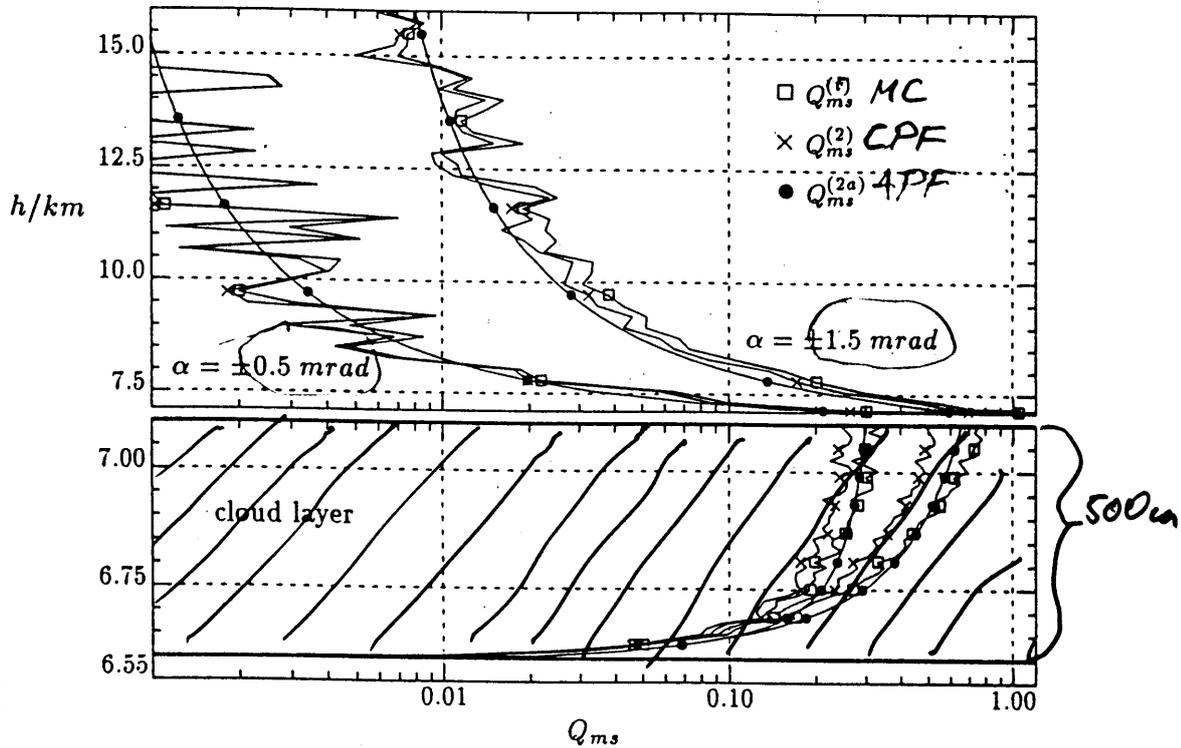
Figure 6: Same as Figure 4, showing the  $Q_{ms}$ -approximations as a function of the height  $h$  for water droplet clouds at the height of 7 km with the optical depth 1.0 using lidar systems with a receiver FOV angle  $\alpha = \pm 0.5 \text{ mrad}$  (left group of curves) and  $\alpha = \pm 1.5 \text{ mrad}$  (right group of curves).
