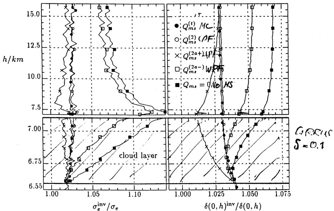
Figure 10: Same as Figure 7, except that the inverted signals were simulated using a ice crystal cloud with phase function No. 1.1 of Table 1 at the height of 7 km with an optical depth 0.1.
