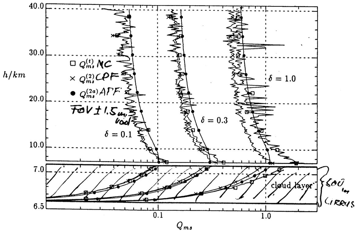
Figure 5: Same as Figure 4, showing the  $Q_{ms}$ -approximations as a function of the height  $h$  for ice crystal clouds at the height of 7 km using lidar systems with a receiver  $FOV$  angle  $\alpha = \pm 1.5$  mrad.
