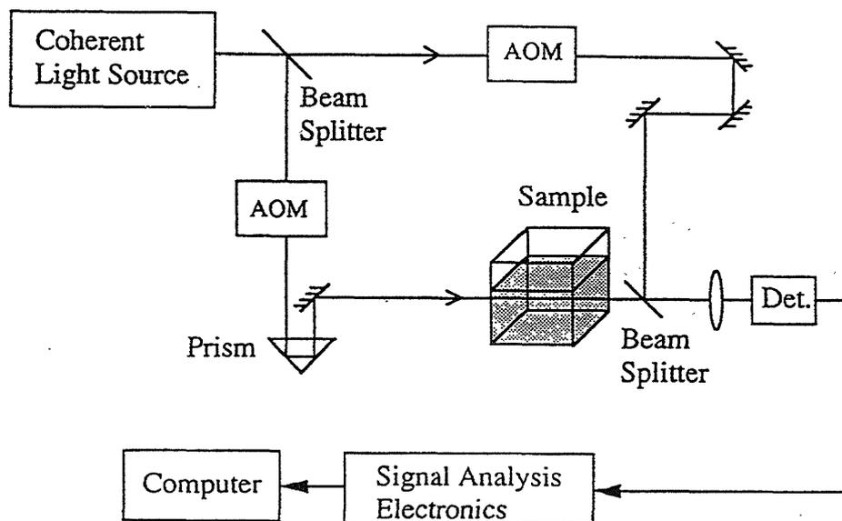
Fig. 1 Schematic diagram of the coherent detection imaging (CDI) system.
