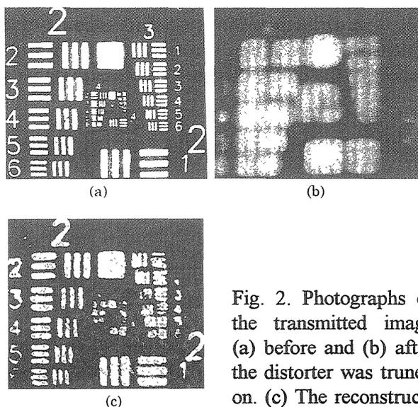
Fig. 2. Photographs of the transmitted image (a) before and (b) after the distorter was turned on. (c) The reconstructed image.
