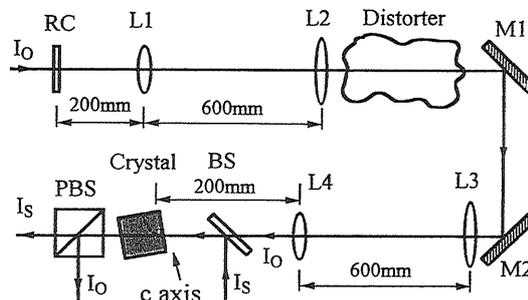
Fig. 1. Schematic of the experimental setup. Lenses L1 and L4 have a focal length of 200 mm; lenses L2 and L3 have a focal length of 400 mm. M1, M2, mirrors. Other abbreviations are defined in text.
