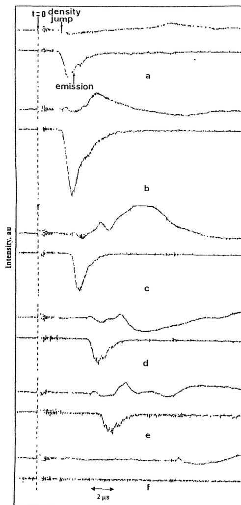
Fig. 2. Time history of the density jump and plasma emission taken at various position from the glass target in air at 100 torr. a) 1mm, b) 2mm, c) 3mm, d) 4 mm, e) 5 mm and f) 10 mm.
