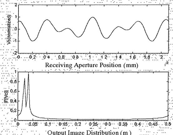
Fig. 4 Simulated result for the same conditions as in Fig. 3. Correlator output function ( top ), and its Fourier transform ( bottom )
