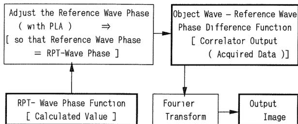
Fig. 2 Block diagram of the SAILR imaging process using PLA.
