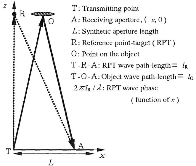
Fig. 1 Concept of 1-D SAILR imaging for static object.
