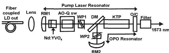
Figure 1 Structure of OPO
