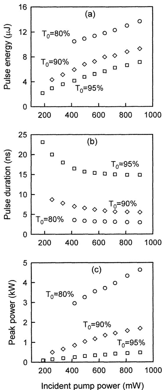
Fig. 2 Pulse parameters versus incident pump power for Cr<sup>4+</sup>:YAG saturable absorbers of initial transmission  $T_0 = 80\%$ ,  $90\%$  and  $95\%$ , respectively. (a) Pulse energy, (b) Pulse duration, (c) Peak power.
