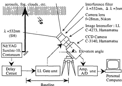
Fig. 1 Bistatic imaging lidar system
