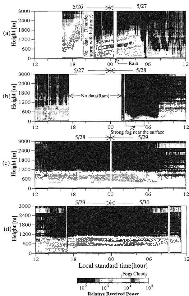
Fig.2 Time-height representations of the laser return signal intensity measured at Moriya from noon May 26 to noon May 30,1997.
