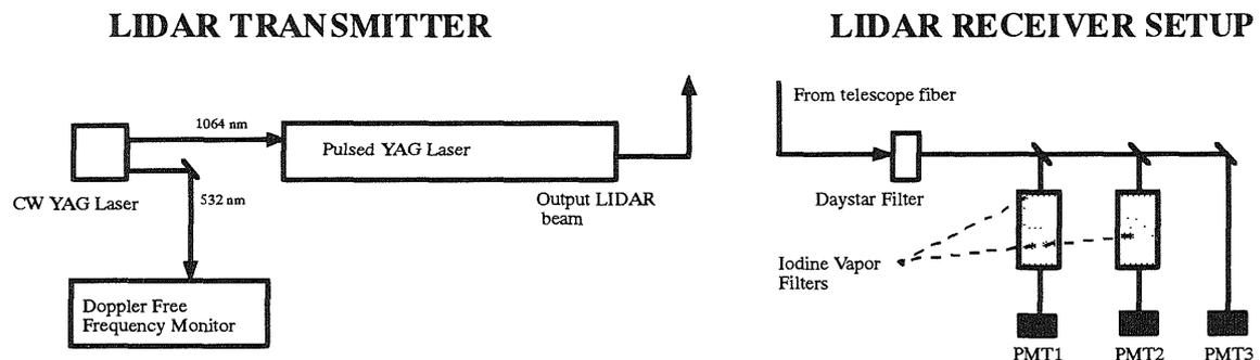
**Figure 1.** Schematic of the HSRL system. The transmitter system consists of a seeded pulsed YAG laser of 74 MHz linewidth. The receiver consists of two molecular and one total scattering channels.
