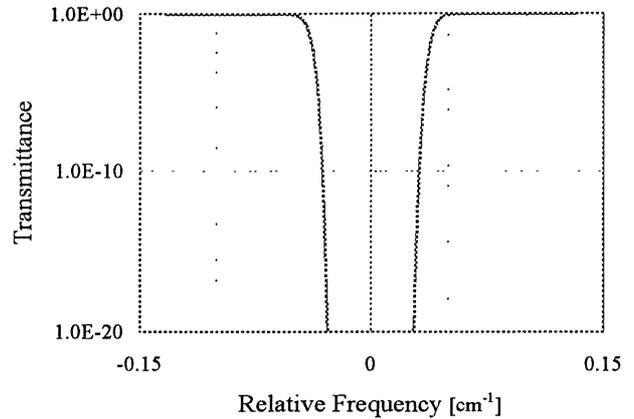
Fig.5 Transmittance around the resonance frequency of Cs filter. Cs atomic parameters are given by Table1.
