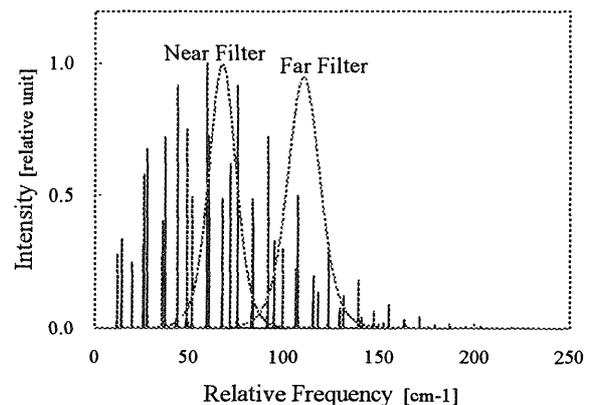
Fig.1 Calculated distribution of the intensity of the rotational Raman line backscattered by atmospheric molecules (at 255[K], 5[km]), and position of the filters. (The center frequencies of the near and far filters are 68 and 107  $cm^{-1}$  from the laser frequency, respectively. The bandwidths of the near and far filters are 19 and 22  $cm^{-1}$ , respectively. The laser frequency is 25716 $cm^{-1}$ .)
