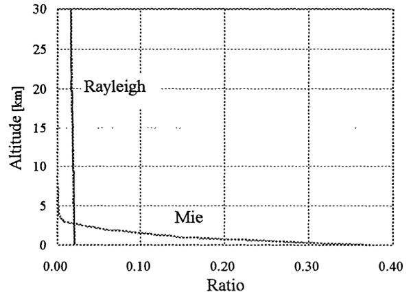
Fig.4 The ratios of the intensities of the Rayleigh and Mie scattering, respectively to Raman scattering intensity transmitted through the near filter up to 30km under the condition of the U.S. Standard atmospheric model. (The filter and laser parameters are the same as that of Fig.1.)
