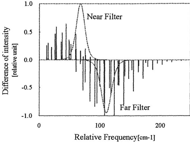
Fig.2 Difference of the intensity of the rotational Raman scattering by atmospheric molecules at temperature between 275 and 255 K in 5 km altitude.
