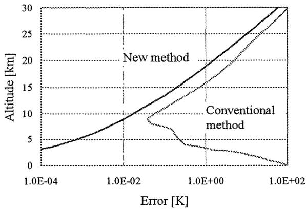
Fig. 7 Accuracy profiles of the two methods up to 30km.
