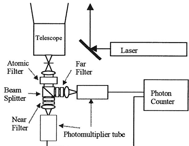
Fig. 6 Scheme of the rotational Raman lidar using the atomic filter and the interference filters.
