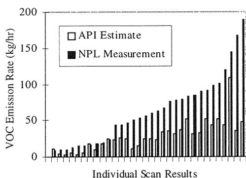
Figure 3. Comparison of NPL DIAL results and API estimated emissions
