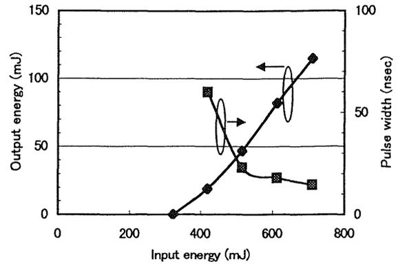
Figure 4-1 Input and Output Characteristics under Ordinary Temperature and Atmospheric Pressure
