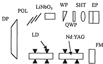
Figure 3-1 Block Diagram of Laser Oscillator
