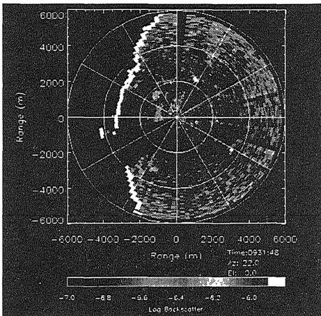
**Ground and Ambient Backscatter Removal**
