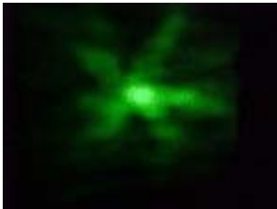
Fig. 2 Example of LRNB generation using 20cm diameter telescope and 0.53 \mu\text{m} Nd:YAG laser. The picture was taken at 4.5km distance. The central bright spot corresponds to LRNB.
