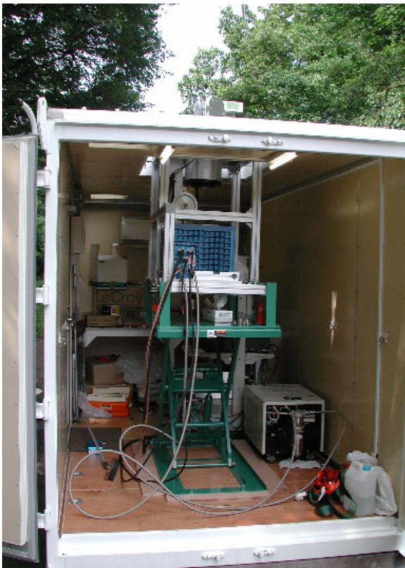
Fig.2 (left) 2-axis coherent Doppler lidar. Installed in a container for lidar observations. The lidar is lifted by a electrical lifter during observations, and it is stored at the end of observations. (right) exterior of a 2-axis waterproof scanning system.
