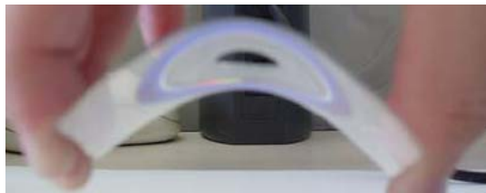
Fig.3 The elasticity of an optical memory card
