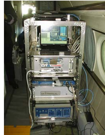
Figure 1. Airborne 2μm coherent Doppler lidar
