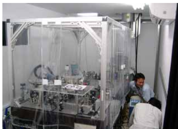
Fig.1 (Upper) exterior of a lidar container and a 2-axis waterproof scanning system, and (lower panel) 2-axis coherent DIAL Installed in a container for the lidar measurement.
