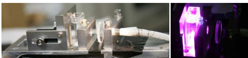
Fig. 1 Quartz cell holder used for the LIF measurements. The right panel shows the bright feature of the cell during the UV laser irradiation.
