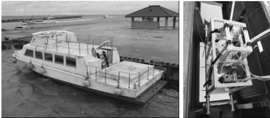
Fig.3 Photographs of the glass-bottom-boat and the fluorescence imaging lidar on the boat.
