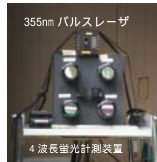
Fig.1 Fluorescence imaging LIDAR
